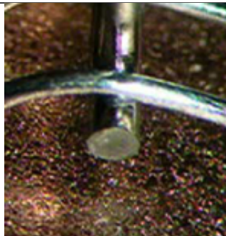
Thick aluminium wire pull test
