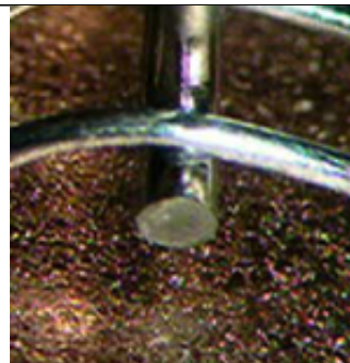
Thick aluminium wire pull test
