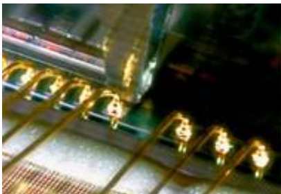
Figure 1: shear testing of gold ball bonds within a semiconductor device
