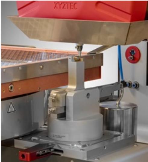
With the high accuracy bond tester comes a sample carrier and cooling down rack to make the handling of the large (hot) panels easy. The carrier can be positioned accurately before testing and then safely cool down after the automatic tests.
