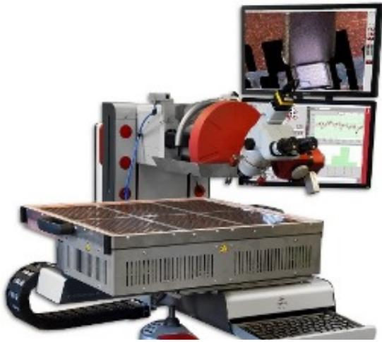
XYZTEC has historically been very successful in working together with customers to develop customized solutions for new quality assurance challenges in a highly competitive world. This case study describes the solution XYZTEC found in order to enable a customer to test glued or solder interconnections on a coating at temperatures up to 175°C.
