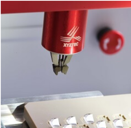
Highly reproducible stud pull tests by using the Sigma as a pick and place machine
