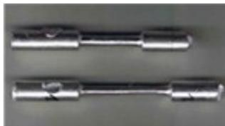
During the tensile test the samples will be extended with a constant rate until fracturing. The result of such material testing for a BiSnAg-solder is shown in figure 9 as an example.
