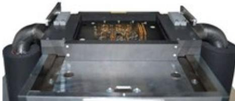
**Figure 12 - Test adapter (lower part) in heated test handler - the tubes from the side transport**
