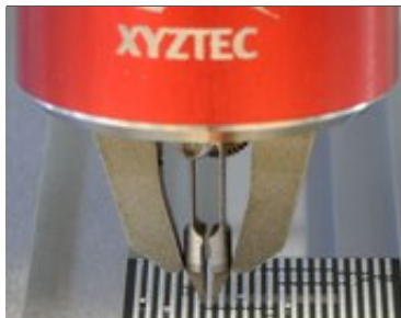
USB Tweezers performing cold bump pull (CBP)
