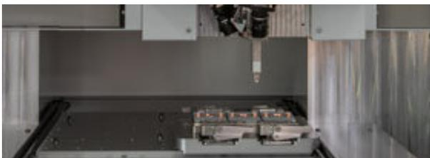
Most rigid test head in the industry for forces up to 1000 kgf.
