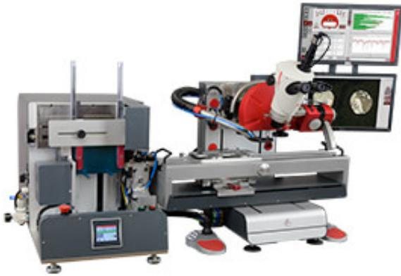
Condor Sigma MAG is a fully automatic magazine handler for lead frame testing
