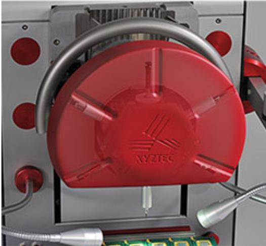
Six sensors RMU, up to 200 kgf: changing cartridges manually no longer required
