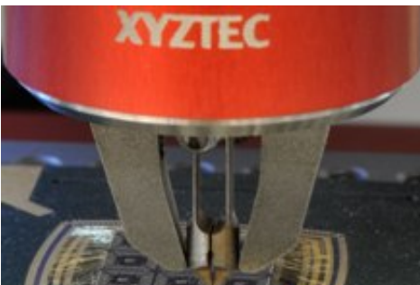
Exchange tips of USB Tweezers within seconds
