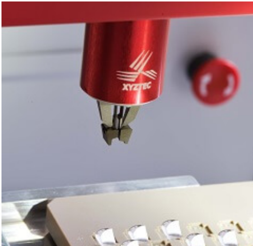
Highly reproducible stud pull tests by using the Sigma as a pick and place machine
