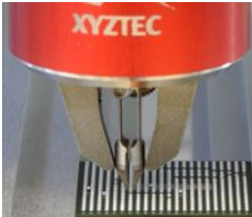
USB Tweezers performing cold bump pull (CBP)
