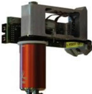
When mounted on a Condor Sigma pull sensor, you can detect touchdown on your sample
