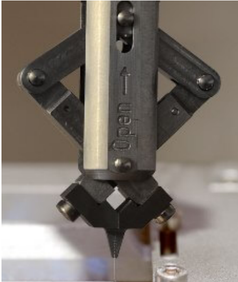
Mechanical tweezer for forces up to 50 kgf
