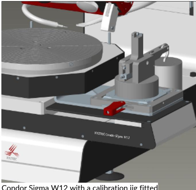
Condor Sigma W12 with a calibration jig fitted
