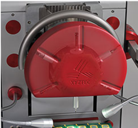
Six sensors RMU, up to 200 kgf: changing cartridges manually no longer required
