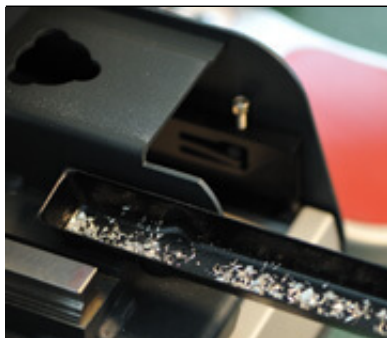
Debris is kept away from the moving parts without the need for sliding seals
