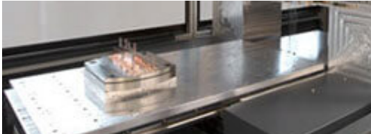
Extra large working area of 500x800x200 mm
