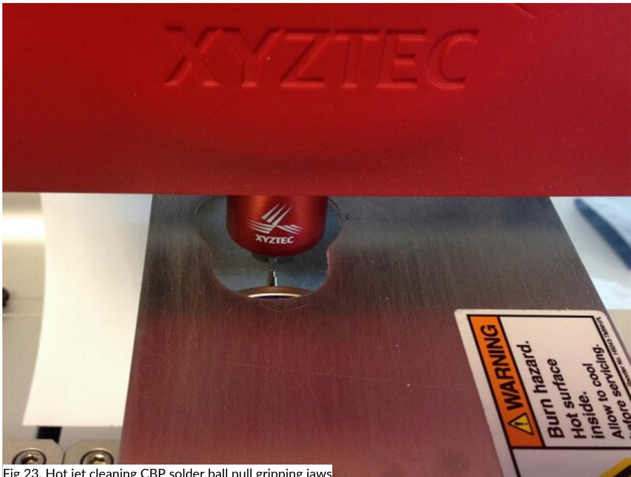
Fig 23. Hot jet cleaning CBP solder ball pull gripping jaws
