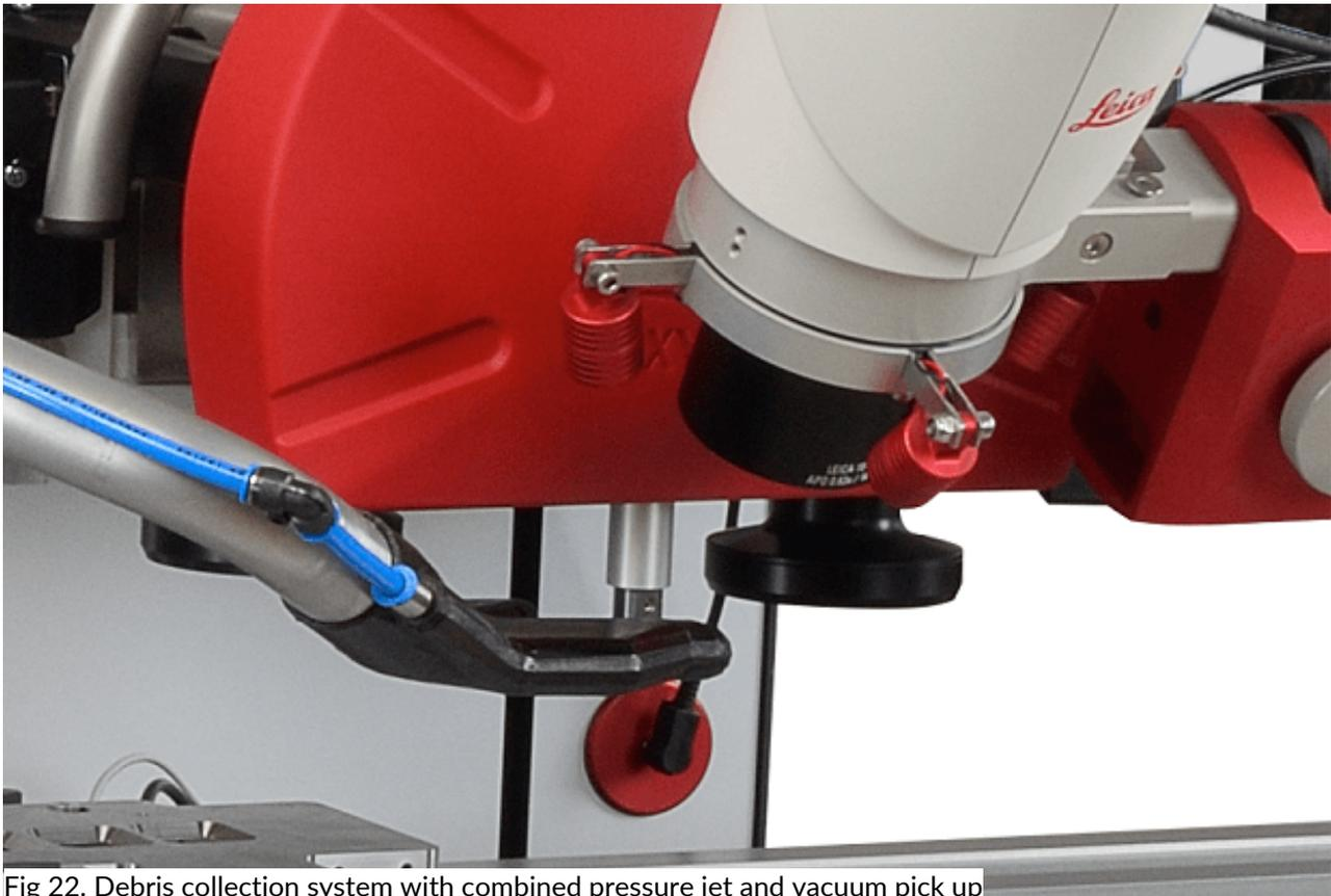
Fig 22. Debris collection system with combined pressure jet and vacuum pick up
