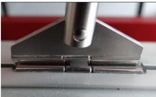
Uni-axial bending test performed on Condor Sigma
