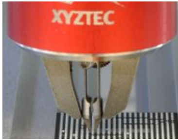
USB Tweezers performing cold bump pull (CBP)
