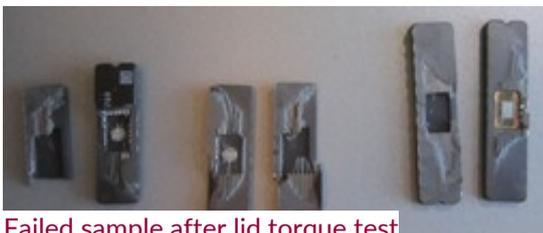
Failed sample after lid torque test
