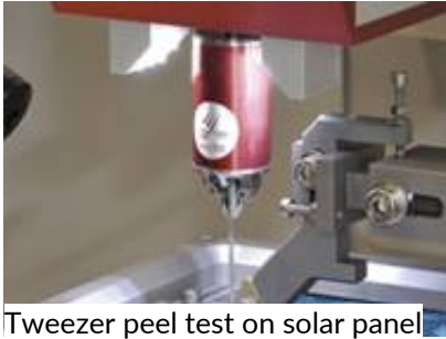
Tweezer peel test on solar panel
