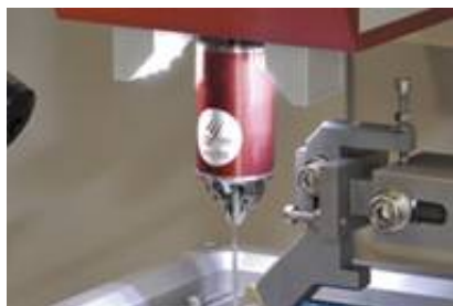
Tweezer peel test on solar panel
