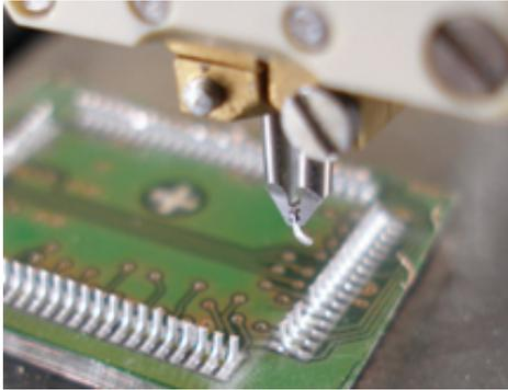
IC lead peel test
