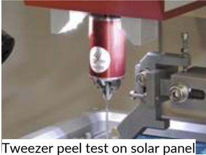
Tweezer peel test on solar panel
