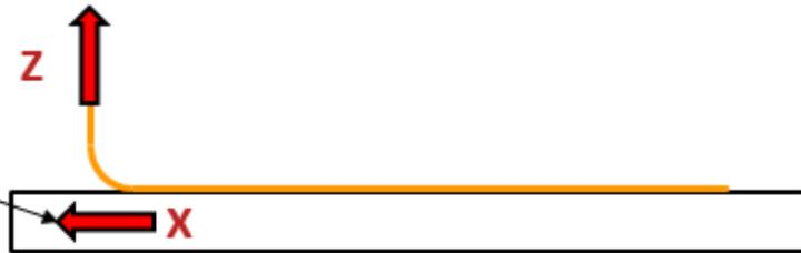
Apart from the peel radius the **Peel Point** remains under the **Peel Line**
