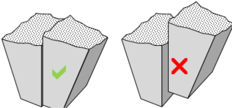
Misalignment of the jaws must not influence the failure mode of interest or the test force
