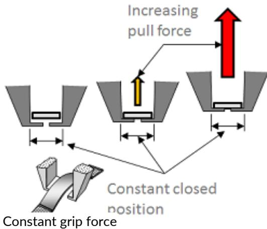
A constant grip force regardless of the increasing pull force is useful when gripping soft parts, where the sample can be deformed to obtain a grip but squashed too much if the grip force gets too high.
