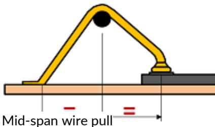
We also have to align the hook along the length of the wire; where do we pull? Common practice is to pull at the center of the wire. The **MIL standard 2011** specifies pulling between midspan and loop apex in order to avoid adverse wire deformation (previous versions of the same standard specified pulling mid span).
