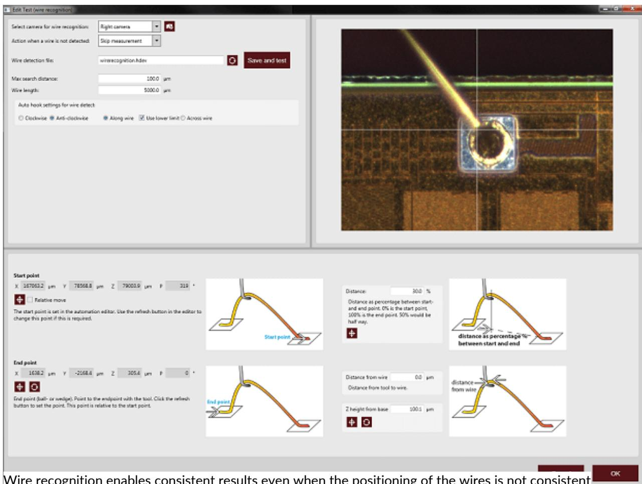
Wire recognition enables consistent results even when the positioning of the wires is not consistent
