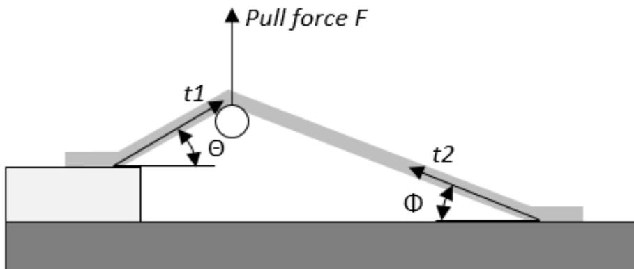
In DVS 2811 the pull alignment position is made so  $\theta = \phi$ .
