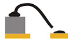
Heel strength known Acceptability depends on strength
