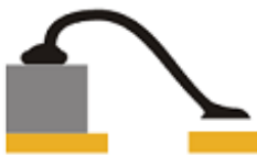
Wedge bond Wedge bond strength known Acceptability depends on strength
