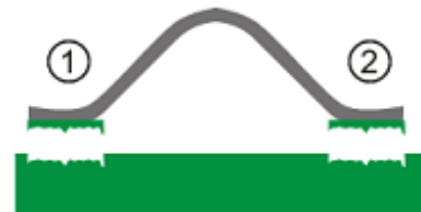
Both wedge crater Probably weak bonds Possibly bonder process problem
