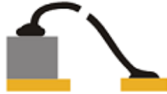
Mid span Bond strength unknown Acceptability depends on strength
