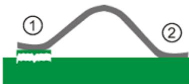
Wedge crater Acceptability depends on strength Possibly bonder process problem
