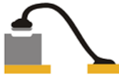
Pad crater Pad strength known Acceptability depends on strength Possibly bonder process problem
