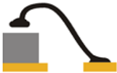
IMC/Bond strength known Acceptability depends on strength
