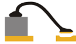
Wedge crater Acceptability depends on strength Possibly bonder process problem
