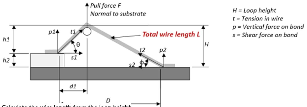
Calculate the wire length from the loop height
