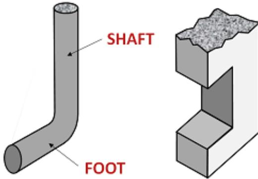
Most hooks are made from bent round wire. Special machined hooks of any shape are also available.
