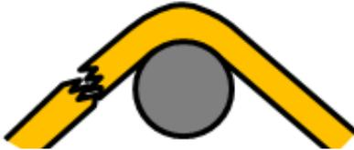
The wire hook diameter should be around 3X the wire diameter to avoid cutting the wire
