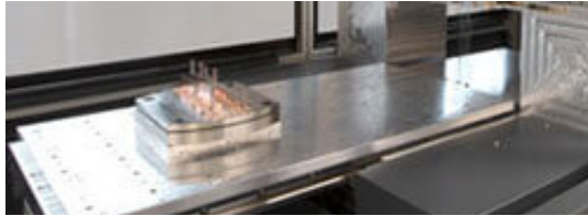
Extra large working area of 500x800x200 mm
