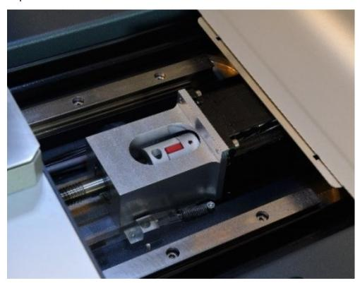
The Sigma direct drive motor and linear encoder ensure ±1µm accuracy.
