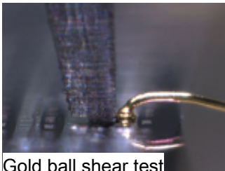
Gold ball shear test
