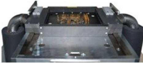
**Figure 12 - Test adapter (lower part) in heated test handler - the tubes from the side transport**
