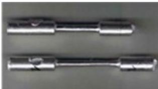
During the tensile test the samples will be extended with a constant rate until fracturing. The result of such material testing for a BiSnAg-solder is shown in figure 9 as an example.
