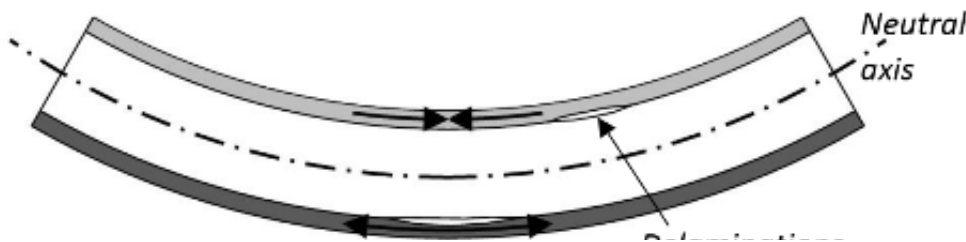
Delamination can occur when bend testing. Picture courtesy of Fraunhofer institute
