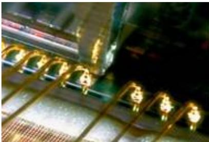
Figure 1: shear testing of gold ball bonds within a semiconductor device
