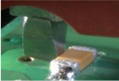
Figure 2: impact measurement unit testing chip capacitor mounted on printed circuit board
