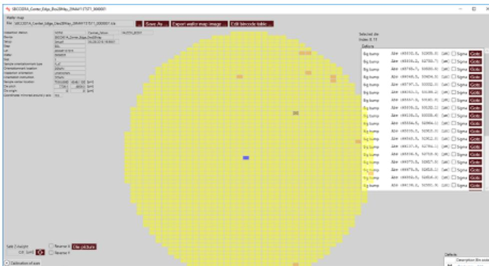
The wafer map control screen, offers import of multiple wafer map file formats and shows defects and tested positions
