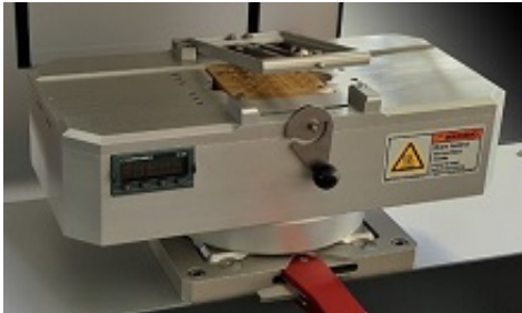
Heater workholder (up to 500°C) mounted on the Sigma by quick release system
