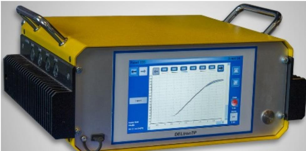
Windows based temperature controller with various heating profiles for Condor Sigma W12 Cooling down rack
