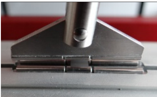
Uni-axial bending test performed on Condor Sigma
