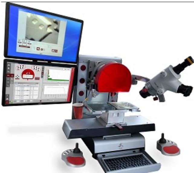
Highly reproducible stud pull tests are possible
