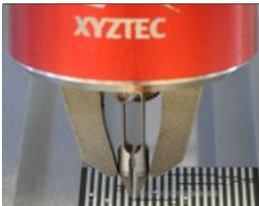
USB Tweezers performing cold bump pull (CBP)
