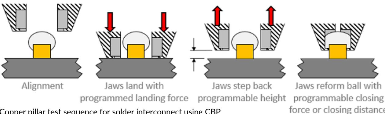
Copper pillar test sequence for solder interconnect using CBP
