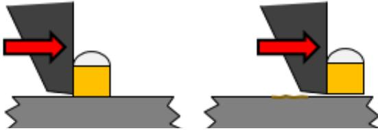
Copper pillar low shear height and bond fails in shear
