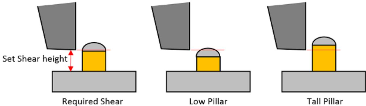
Tolerance build up can cause problems when shear testing the copper bump using conventional methods
