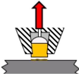
Pull test copper pillar gripped with two tapered cavities
