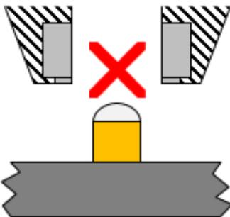
The solder interconnect is very difficult to test. Shear is the best test
