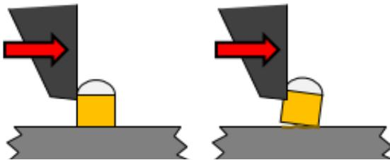
Copper pillar high shear height and bond fails in tension
