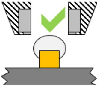
This shape of solder is possible to test similar to regular Cold Bump Pull (CBP)
