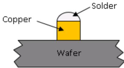
The Condor Sigma can test copper pillars down to 35µm diameter
