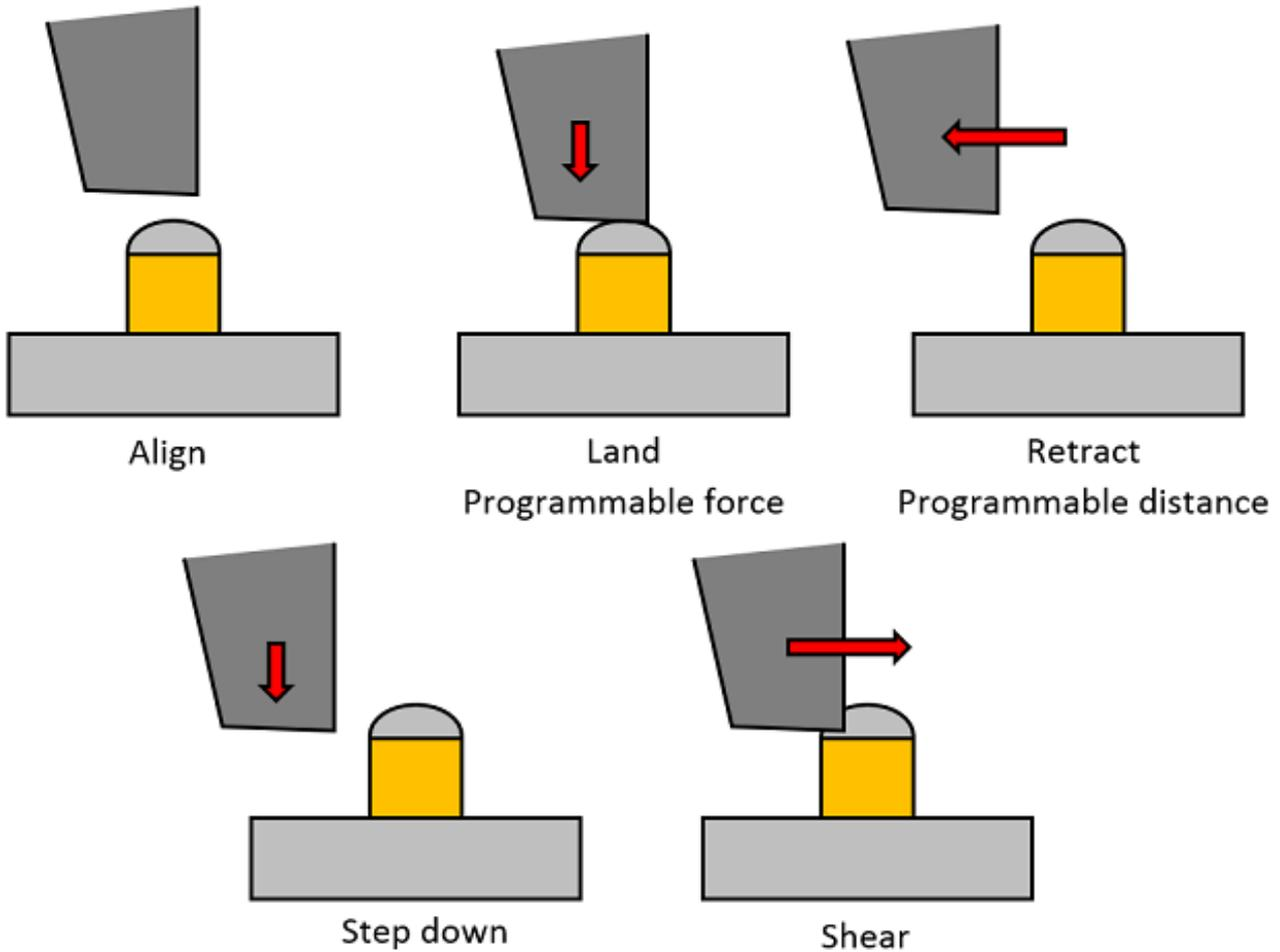
The test sequence using XYZTEC's unique top landing shear method
