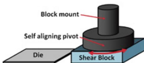
The self aligning shear tool is designed for forces up to 500kgf
