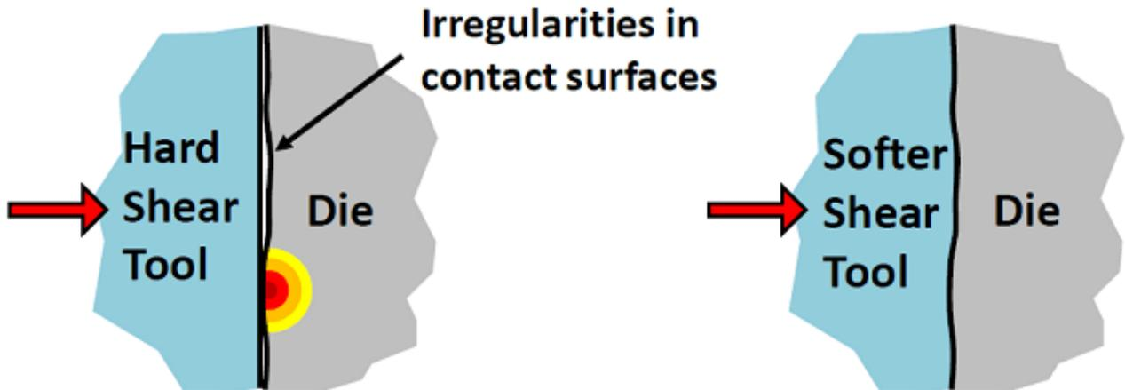
XYZTEC discovered that it is often better to use a shear tool made of a relatively soft material when performing high force die shear
