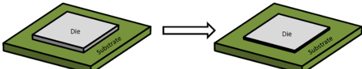
There are three aspects of these designs that make testing difficult. Firstly, the reduced ratio of die thickness to die bond area, shown in this illustration. Secondly, die and substrate warpage can be a problem. And thirdly, the bond strength is often very high, for example when silicon is bonded directly to silicon or other similar materials.
