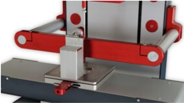
XYZTEC designed a special work holder for lead integrity testing. It is available for the Condor Sigma and Condor Classic platforms. Shown here is the Condor Sigma version.
