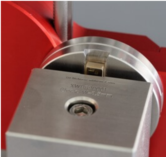
Detail of the lid torque workholder on a Condor Sigma
