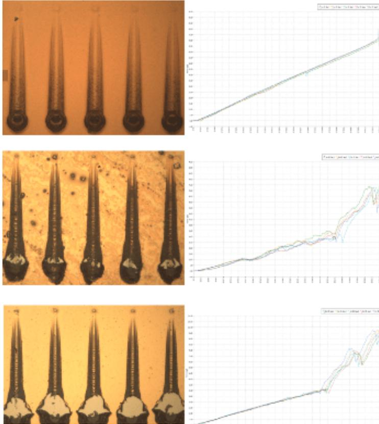
These examples show the same Progressive Load Scratch Test (PLST) on multi layer films of different constructions
