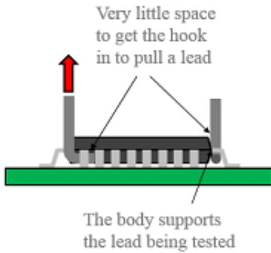
Straightforward pull testing on SMD Gull Wing Leads has two main disadvantages
