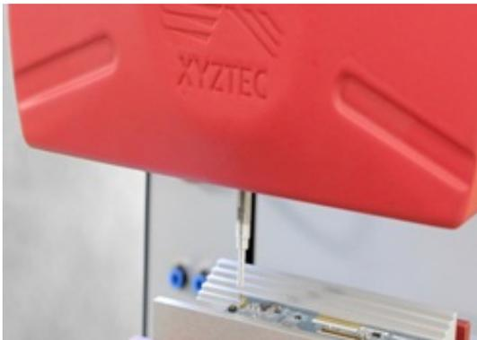
Our test platforms have auxiliary inputs for external sensors, which can be very useful during spring rigidity testing
