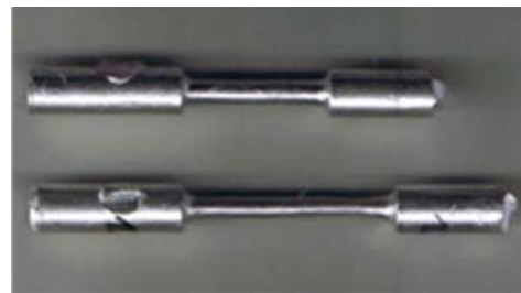
Figure 8. Typical solder samples for tensile testing (before and after testing)
