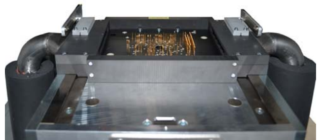
Figure 12. Test adapter (lower part) in heated test handler - the tubes from the side transport the heated air [MOE-12]
