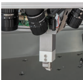
Unique 360° head design with up to five mounted cameras
