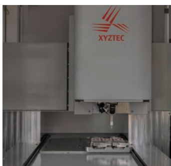
Most rigid test head in the industry for forces up to 1000 kgf.
