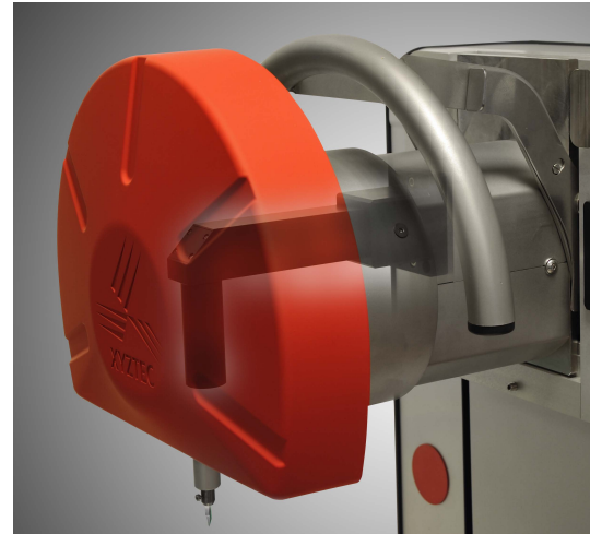
Partially transparent Condor Sigma measurement unit showing the integrated camera solution
