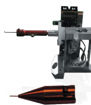
Modular Pull sensor: Use existing pull tools
