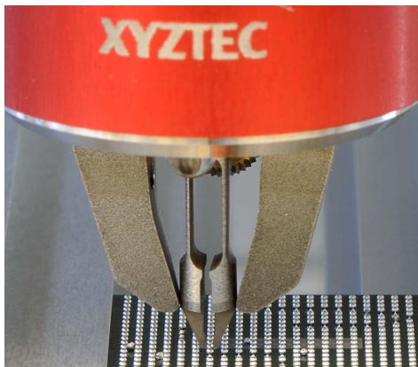
XYZTEC USB Tweezers gripping a solder ball
